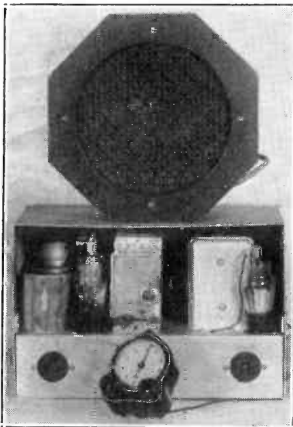
The de luxe car radio — the Supertone "Wanderlust"—uses a perfected remote control unit, a tone-quality speaker, and the latest tubes.
